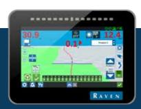
The CR7 is a 7-inch lightweight field computer with customizable in-job layouts. A simple widget concept, easily accessible settings, and ISO Universal Terminal and Task Controller capabilities make this mighty unit an affordable, plug-and-play system.
