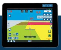
The CR12 is the latest field computer in the CRX display family, joining the CR7. Uniquely, the CR12 offers an extensive field planning feature, allowing the user to define AB-lines and reference lines of the field boundary. The user can then setup the complete field, including multiple headlands, spray tracks, greening zones and tracks with different working widths.
