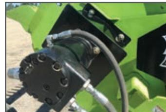
The direct drive motor has a built in cushion valve
