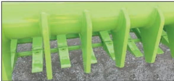
450 BNH steel for heavy duty windrowed picking
