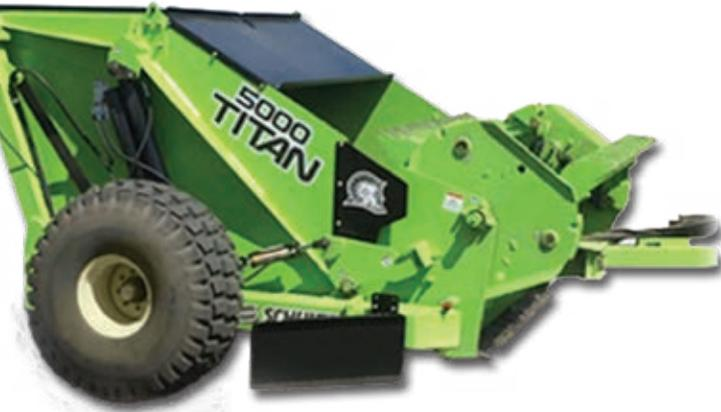
Spend more time picking and less time dumping with the enormous Schulte 5000 Titan Rock Picker. The huge 5cu yard bucket is actual stone picking capacity. The Titan also features a 6.5' tall dump height for larger rock piles and for truck loading.
