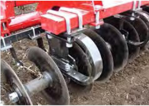
Disc gangs are protected by the mounted C-spring to absorb shock by field obstructions.
