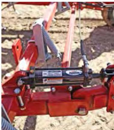
A weight transfer kit is available for the QX<sup>2</sup> and is standard on units with 5- and 6-foot (1.5 and 1.8 m) outer wings, as well as 5-section units. The kit is optional on all other models. This kit puts weight on the floating hitch and the front gauge wheels to create more stability during transport.
