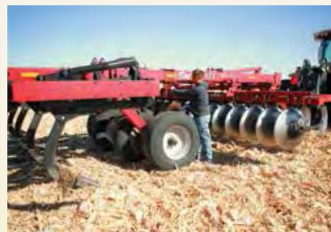
Heavy-duty 4 x 8-inch (10 x 20 cm) frame adds additional weight to keep the tool in the ground and ripping through even the heaviest residue.
