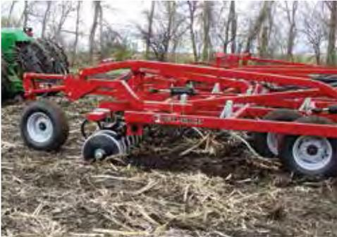
Depth control on 4-foot (1.2 m) wings is maintained by a rigid outer gauge wheel. 7-foot (2.1 m) wings have a single wing axle with hydraulically controlled, front-mounted castoring gauge wheels. Units with 10-foot (3 m) wings have tandem axles with hydraulically controlled front-mounted castoring gauge wheels.
