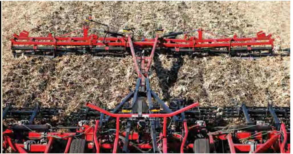
The Rolling Packer finishing attachments leave your field firm and smooth. Available in both solid round and flat bar configurations, these attachments combine field cultivation and soil packing in one pass. This one-pass solution works well in dry conditions, and the option of using this as a separate pull-behind tool makes the Wil-Rich Rolling Packer a great solution for preparing an ideal seedbed!
