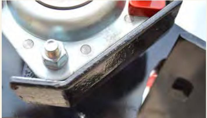
Bearing guard protects bearing from debris.
