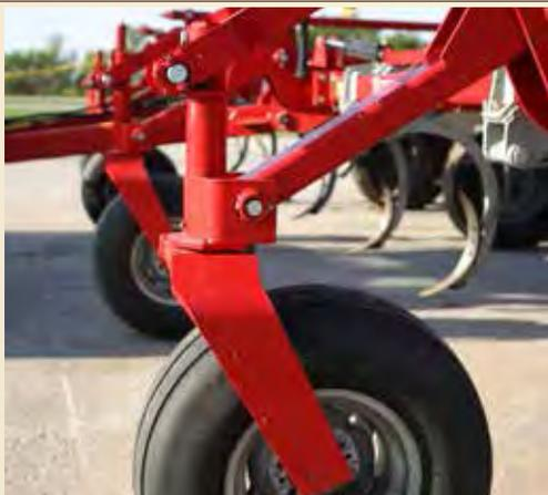
Hydraulic castering gauge wheels are standard on floating hitch models, and ratchet adjust castering gauge wheels are standard on 31-foot (9.45 m) and larger wings.
