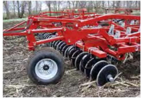
Front-mounted castoring gauge wheels on the wings help maintain stability and consistent working depth.
