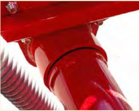
The Wil-Rich 80-foot QX<sup>2</sup> has sealed nongrease axle composite pivots that are virtually maintenance-free.
