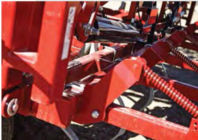
Field cultivators have a rear sixth bar for additional frame strength and more flexibility when mounting finishing attachments.
