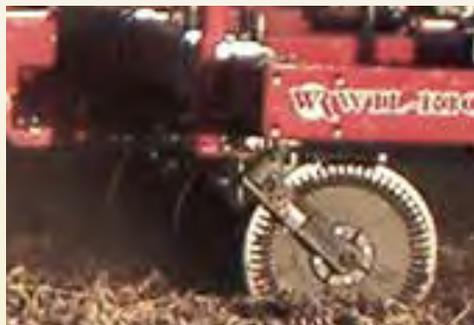
Optional 20-inch (51 cm) spring-loaded coulters easily slice through some of the heaviest residue.
