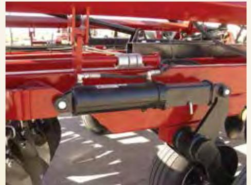
Depth settings are accomplished using simple collars on lift cylinders. There is also optional single-point depth control for easy adjustments.
