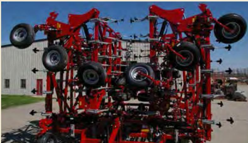
Hydraulic casting gauge wheels carry the unit in the field and lift off the ground and lock into place for transport.
