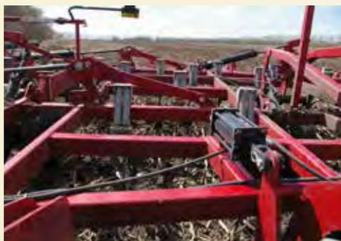
Deep 5-bar frame with 31 inches (79 cm) between ranks allows the Soil Finisher to operate in high residue conditions without plugging. With 125 inches (3.2 m) between the front and rear row of shanks, combined with 9-inch (23 cm) shank spacing, this one-pass disc cultivator is an excellent choice for high residue flow, seedbed preparation, and chemical incorporation.
