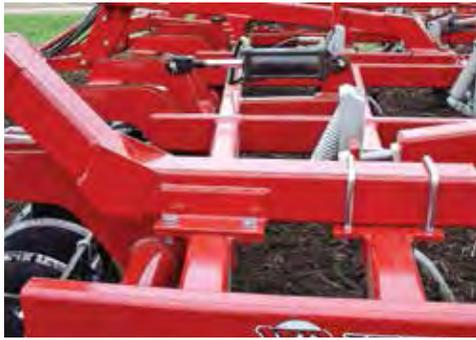
Disc gangs are hydraulically controlled for on-the-go depth adjustments.
