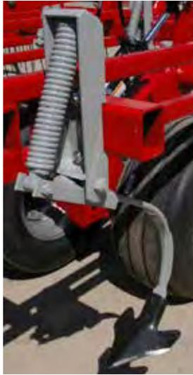
All Wil-Rich shank assemblies are engineered for strength and durability. With edge-on shanks that have wider, zero maintenance pivots designed for the life of the machine and some of the highest trip pressures in the industry, Wil-Rich shank assemblies are the leaders among all categories of tillage equipment. Wil-Rich shank assemblies have plenty of under-frame clearance and are mounted to the machines in a split-the-middle pattern to enhance residue flow through the implement!
