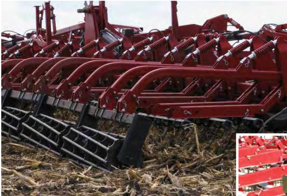
A full complement of finishing harrow attachments is available, including the 3-bar coil tine harrow with round bar basket (shown above).
