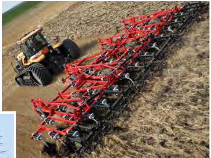
Deep frame is 140 inches (356 cm) front to back, providing superior trash flow for today's higher residue crops.
