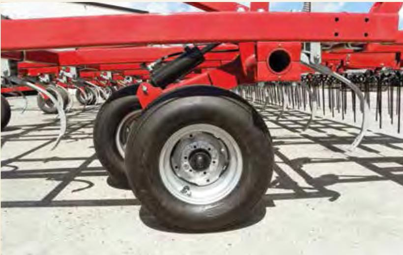
Walking tandems are standard on all main frames and 7-foot (2.1 m) or larger wings. Tire options include 11L x 15 tires or 31 x 13.5 x 15 flotation tires. All units 30 feet (9.1 m) and larger feature 12-ply tires on the main frame. All 5-section units feature highway service tires.
