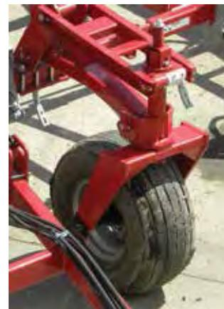
Hydraulic front casting wheels on the main frame of the QX<sup>2</sup> are equipped with a wheel damper kit for stable transport assistance.
