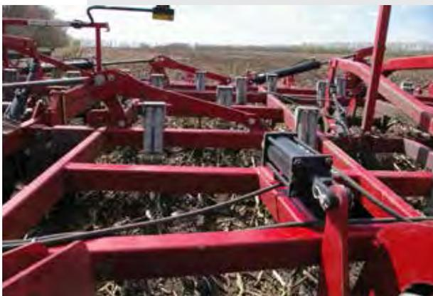
The deep 5-bar frame improves trash flow through the cultivator to maximize tillage and yield.
