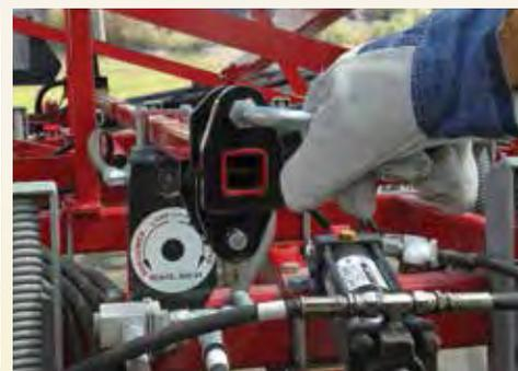
Single-point depth control is a standard feature to allow quick and easy adjustments of working depth.
