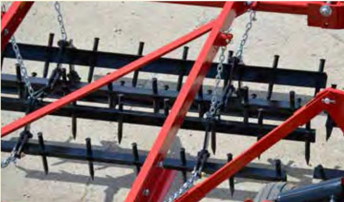
The spike harrow drags the soil and breaks up clods to smooth the ground.
