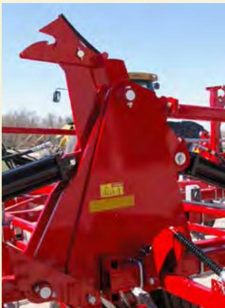
The key to the 80-foot QX<sup>2</sup>'s ability to flex in the field and fold to a relatively small size is the high/low hinge.
