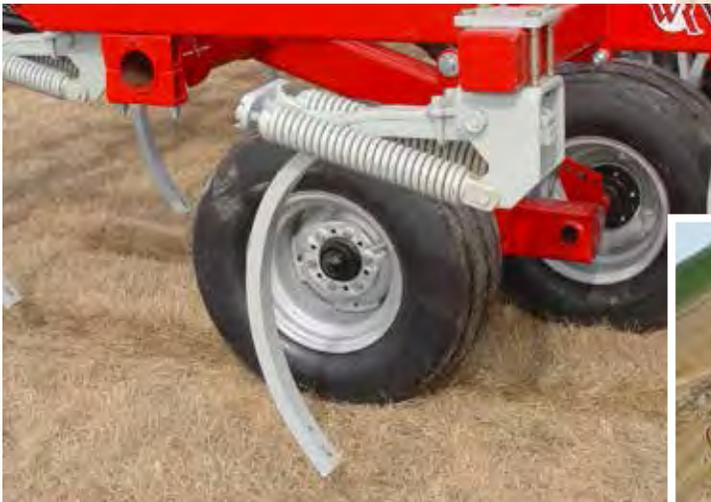
The 650-pound (295 kg) extension spring shank has Wil-Rich's legendary edge-on shanks with wider, zero maintenance pivots that are designed for the life of the machine.
