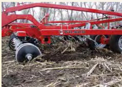
Disc gangs set at an 8-degree cutting angle allow for exceptional cutting and penetration of the 20 (51 cm) x 1/4 inch (.64 cm) shallow, concave blades. Spaced at 9 inches (23 cm), the discs have the ability to penetrate 3 inches (8 cm) deeper than the sweeps and lift to 7 inches (18 cm) above the sweep point. Easily replaceable scrapers work to prevent sticky soil buildup on the disc gang.
