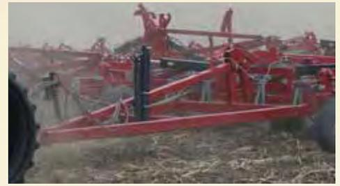
The hitch system features a floating hitch to hug the roughest contours in the field.
