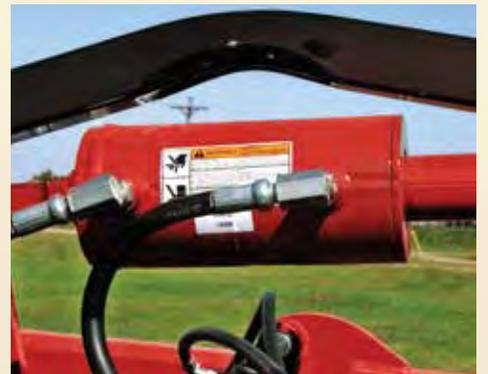
The 614NT Disc Harrow has optional hydraulic leveling.
