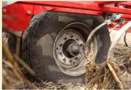
The main frame of the Wil-Rich 80-foot QX<sup>2</sup> rides on four 385/65R 22.5 tires with 10-bolt hubs.
