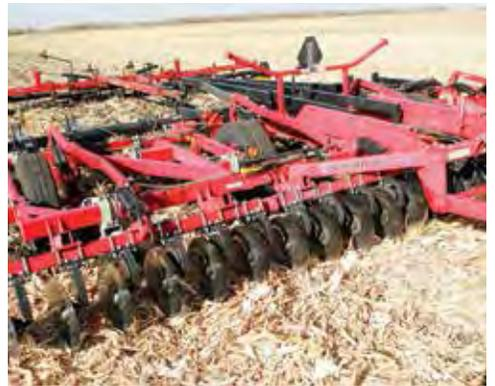
Frame strength and ballast are supported by large, 6 x 4 inch (15 x 10 cm) main frame.
