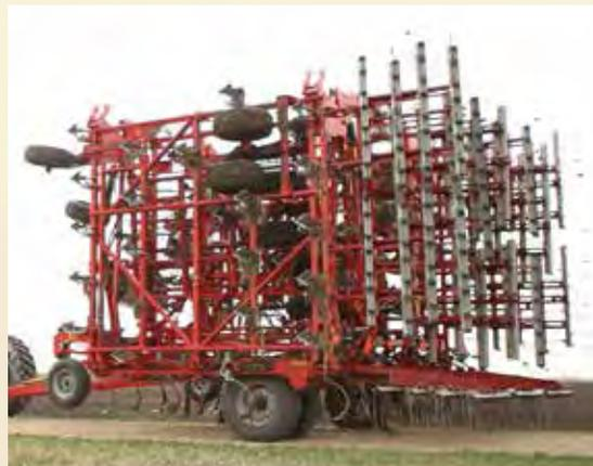
The wings of the Wil-Rich 80-foot QX<sup>2</sup> start in a 90-degree angle to the ground. Both wings unfold. Then the next set of wings unfolds 180 degrees to rest on the ground, and finally one more set of wings unfolds 180 degrees, and the massive Wil-Rich 80-foot QX<sup>2</sup> is ready for work!
