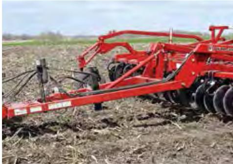
The level lift hitch features heavy 3 x 5 inch (8 x 13 cm) and 4 x 6 inch (10 x 15 cm) tubing with a heavy-duty jack.
