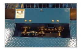
Easy maintenance access to roller chain drive and bearings.
