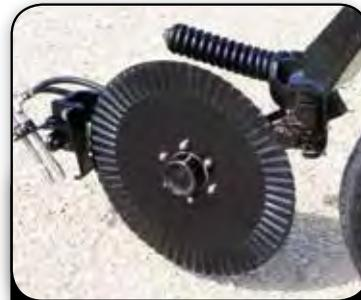
*Six-bolt coulters hubs for extended life*
