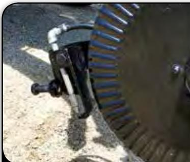
*Injection nozzle or knife injector mounted on heavy-duty 1/2" bar*
